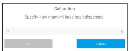
**4.** In the next step you will be choosing the time period after which you would like to be reminded to calibrated the pump again. You will receive notification when there is time to calibrate your pump again.
