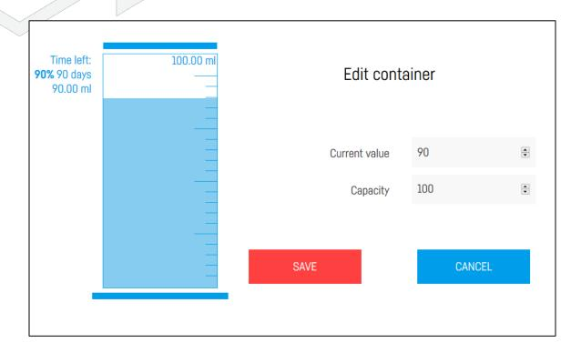
When the amount of liquid inside the container is lower than 10% the device will notify you about this. The notification will be send trough the Smart reef. You can then refill the container with fresh batch of liquid. The "Show more..." button allows for checking the detailed history of the dosing.
