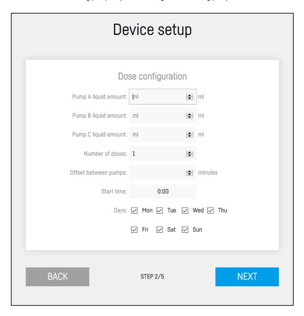
For the dosing pump x3 it is required for safety reasons, to set the delay between each head dosing cycle. It has to be set to prevent the dosing liquids from mixing. The pumps cannot be operating at this same time.
