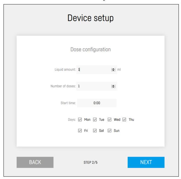
For the Dosing pump x3 you can configure all 3 dosing pumps at once.
