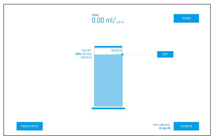
The status screen differs for the Dosing pump X3, that is why we are presenting it separately below. Functionality is this same to the other Dosing pumps. Selecting one of the pumps (A, B, C) will present detailed information about the pump.
