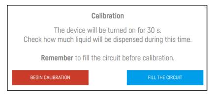
2. The calibration has to be performed right after the initial configuration of the device. Prepare the container that will allow you to measure the amount of liquid (you can use scale, but you might need to know the density of the liquid to calculate the volume). When you have exit of the pump inside the container you can start the calibration procedure. The pump will start operating for 60 seconds.
