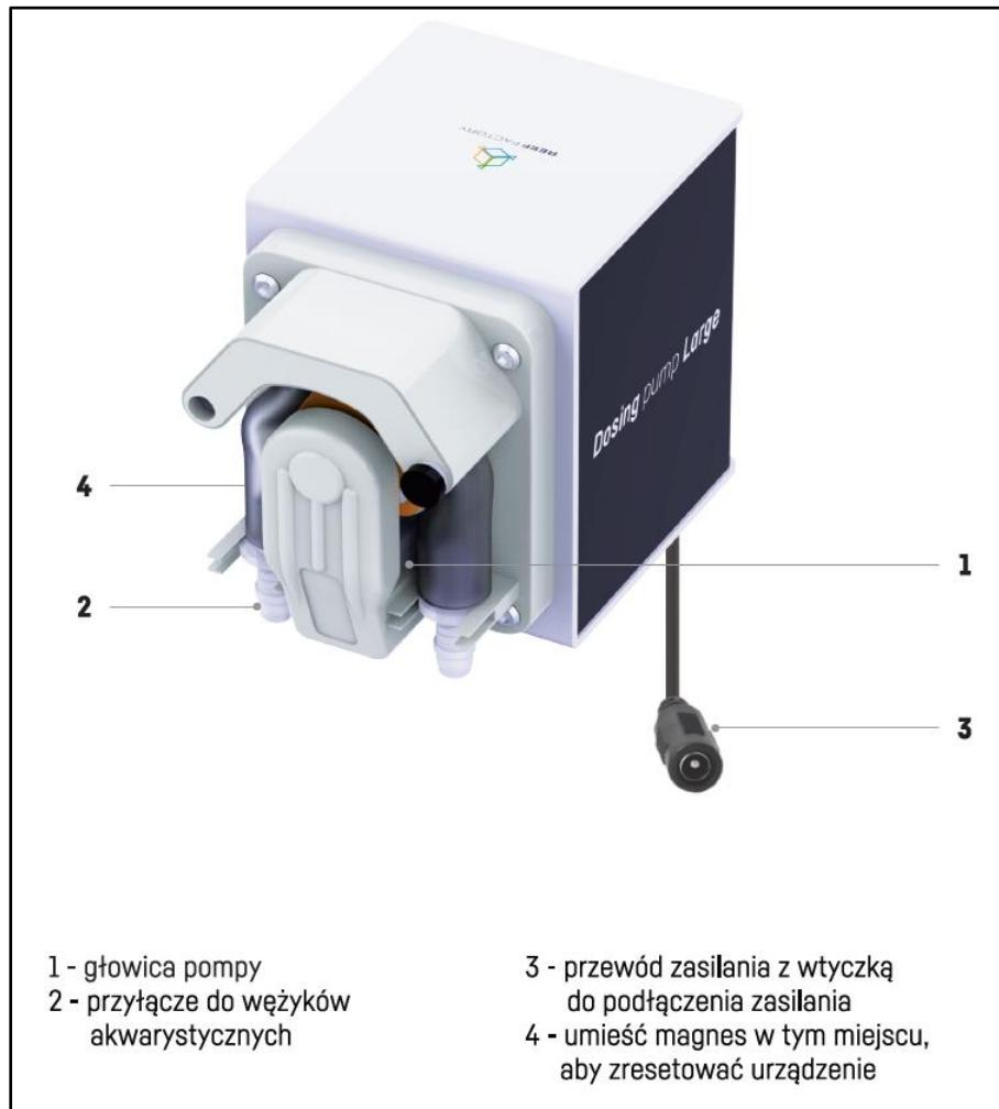
2. Mount the pump head on the pump shaft, cut the silicone tubing to the desired length (remember that they shouldn't be longer than 2 meters as it may influence the dosing accuracy), remove the pump head connector covers and then connect the tubing to the pump heads. Put the other end of the tubing to the container and into the aquarium respectively.
