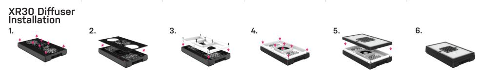
Remove the four corner screws and four fan screws from the lens frame.
